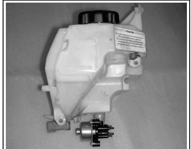
PUMP LOCKED INTO OIL TANK
