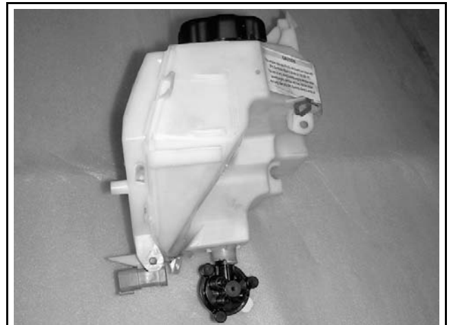
PUMP RELEASED FROM OIL TANK
